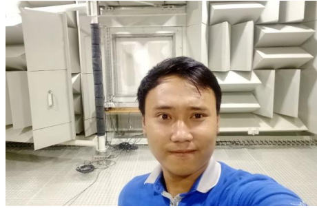
Testing how much sound goes through a wall (the sample is behind Wenda's head)
