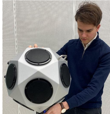
Ben sets up a dodecahedron loudspeaker to create sound going in all directions
